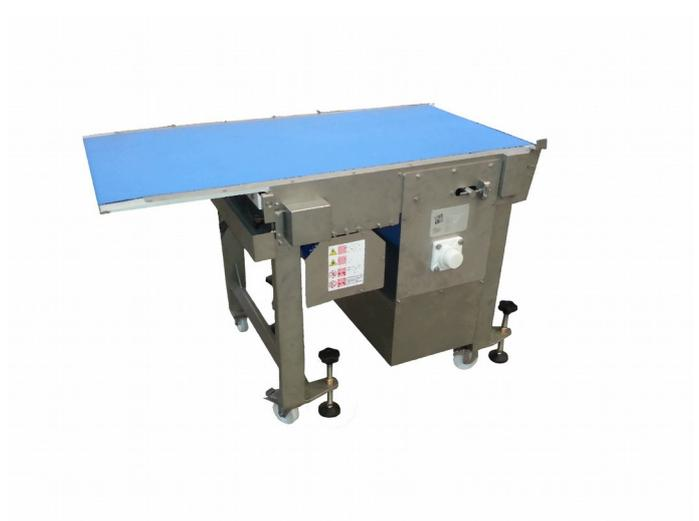
The retractable conveyor (NDS) has been designed to be placed at the exit of the conveyor belt. It's made up by a retractile belt, that discharges the products in transit onto trays. It can also be used to discharge the product on others belts, changing the direction (separating function). Furthermore, the NDS has a device that permits the self-alignment of the belt.
